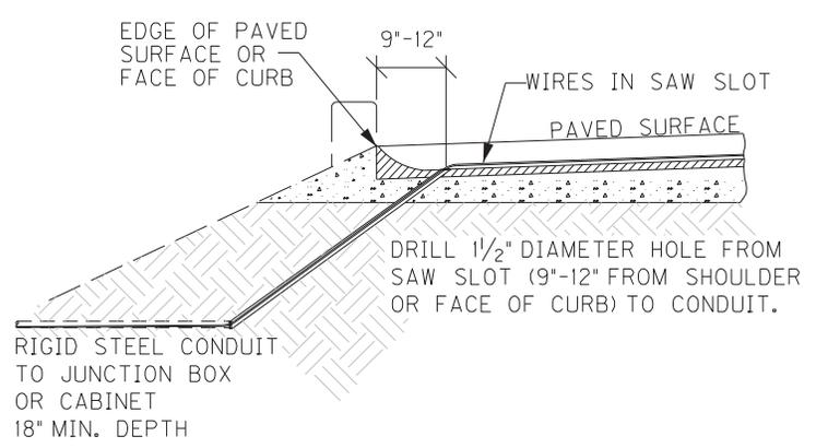
PIEZOELECTRIC SENSOR INSTALLATION
