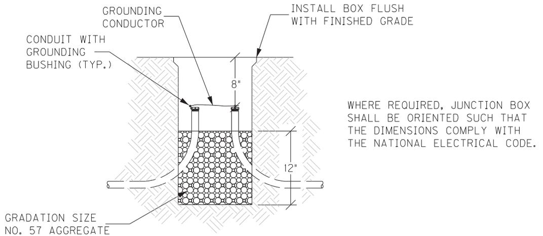
WHERE REQUIRED, JUNCTION BOX SHALL BE ORIENTED SUCH THAT THE DIMENSIONS COMPLY WITH THE NATIONAL ELECTRICAL CODE.
